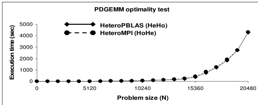
FIG. 5.5. Execution times of the HeteroPBLAS and the HeteroMPI programs on the heterogeneous cluster.  $N$  is the size of the matrix. HeteroMPI program employs heterogeneous 2D block cyclic distribution of matrices.
