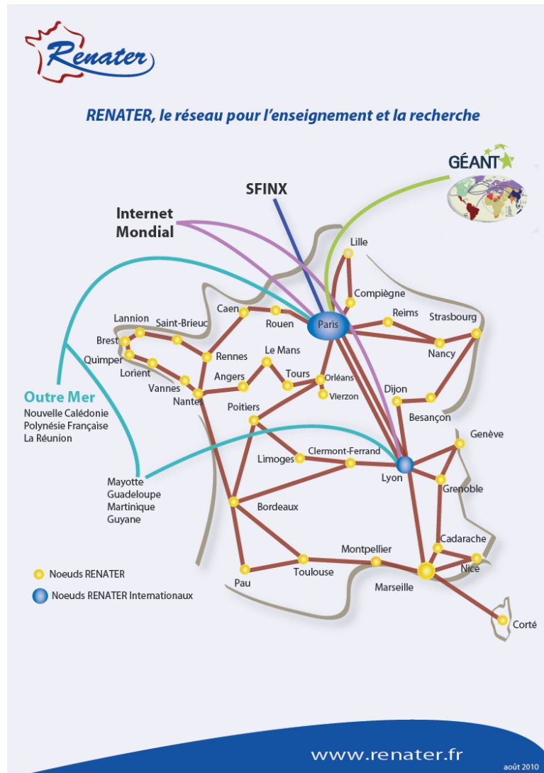
Figure 1.1: The Renater5 Network provides 10Gb/s dark fibre links that Grid’5000 utilizes for its inter-site communication network (Courtesy of www.renater.fr )
